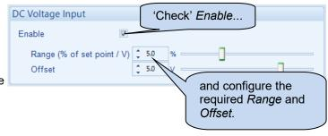
An open circuit input is treated as a 0 V input and so reduces the output voltage to the appropriate percentage of the set point. Using the above example, an open circuit input would reduce the output voltage to 207 V.
